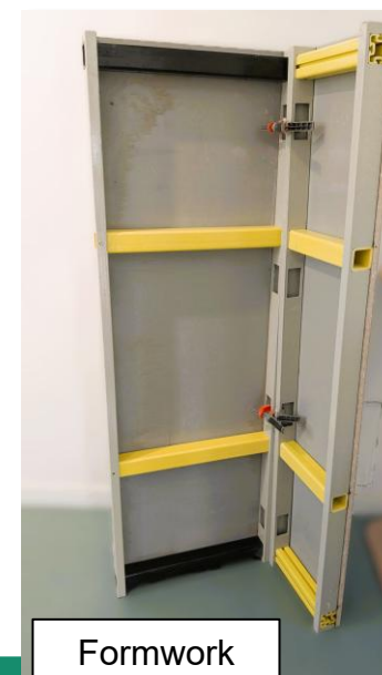
Testing layout of pouring a vertical concrete wall
