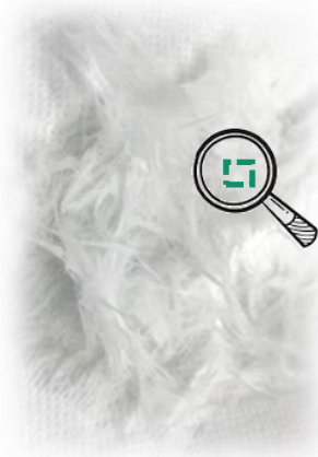
Recovered clean glass fibers without textural damage
