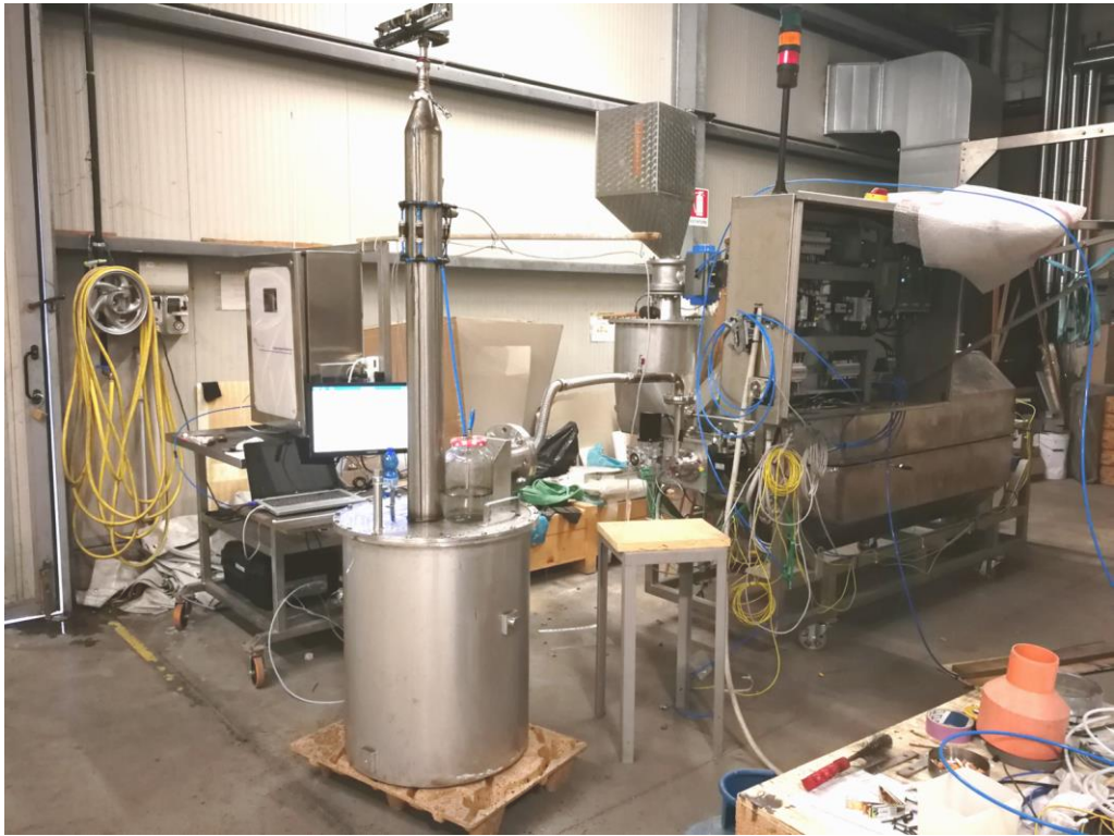
GEOW® continuous reactor, in progress to TRL 5
