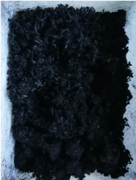
Residual solids, inert, Ø 0 – 0,6 mm = 82 %
