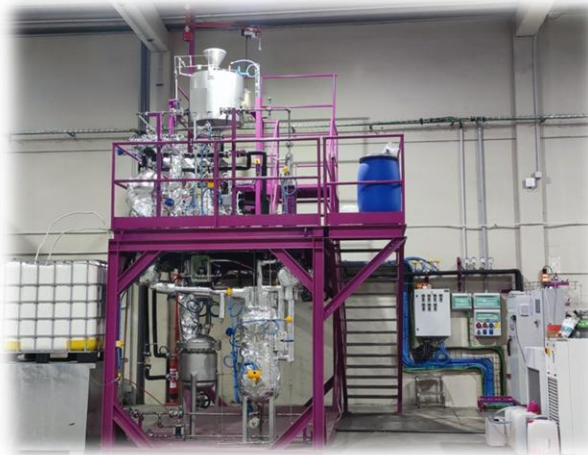
Continuous pilot MW-pyrolysis unit
