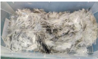
Recycled GF from pyrolysis
