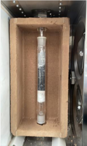
Shredded GFRP & SiC susceptor
