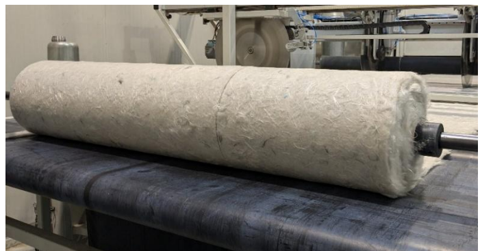
Production of the recycled glass fibre nonwoven mat. (Picture © Cormatex.)
