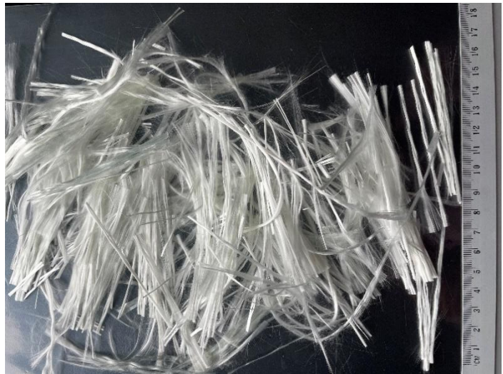
Recycled fibres recovered using Gjenkraft's thermal recycling process. (Picture © Gjenkraft AS.)
