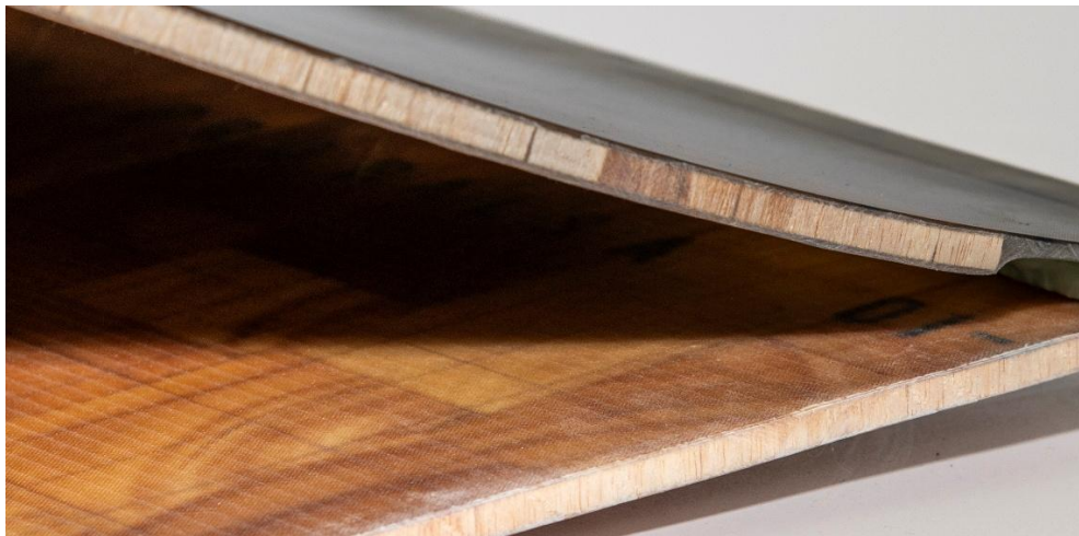
Blade section structure, showing upper shell with recycled glass fibre laminates and balsa core material. (Picture © CETMA / ÉireComposites.)
