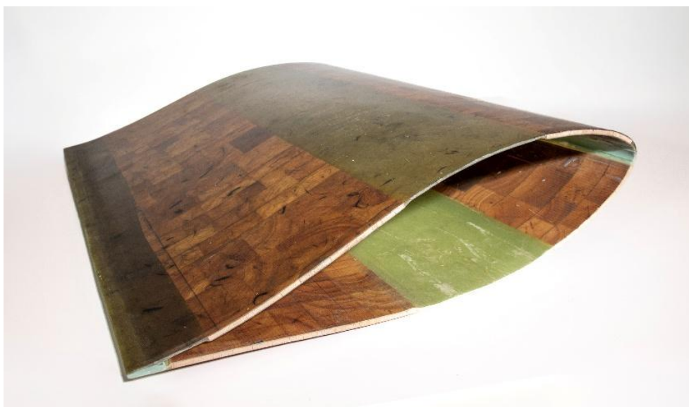
The composite skins of the upper shell of this 1.0 m x 1.5 m blade section were manufactured using recycled glass fibre. (Picture © CETMA / ÉireComposites.)
