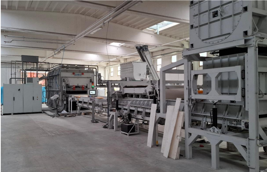
The new Gees recycling line produces panels from blade materials. (Image © Gees Recycling.)
